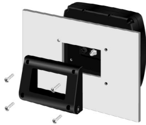
Figure 2-For thin panels, place the mounting bracket on the back side of the panel for additional support.
